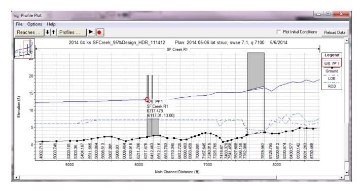
Step 2: The water surface elevation in SFC (including the flow loss contributed by the weirs resulting from step 1) was determined to be 13.0 ft (NAVD).
